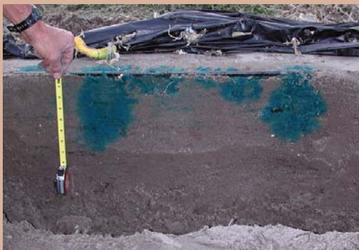
Figure 7. Poor uniformity caused by totally or partially clogged emitters. Photograph by: Eric Simonne.
