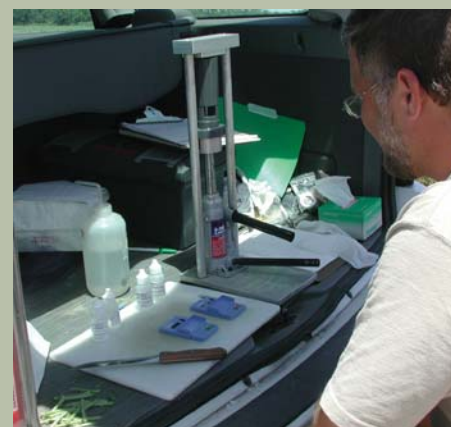
Figure 20. Petiole sap testing may be done in the field shortly after sampling. Photograph by: Eric Simonne.
