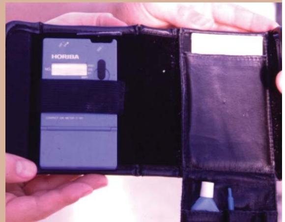
Figure 16. Ion-specific meters are for measuring petiole sap nitrate and potassium concentrations. Photograph by: George Hochmuth.
