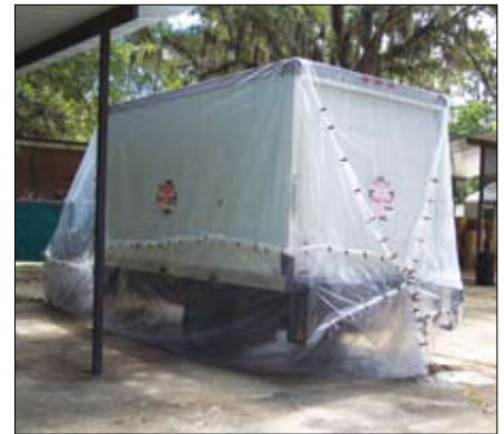
Fig. 4. A truck completely wrapped in 6-mil polyethylene for fumigation of bed bug-infested contents with Vikane gas fumigant. (Photo: E. Hobelmann)
