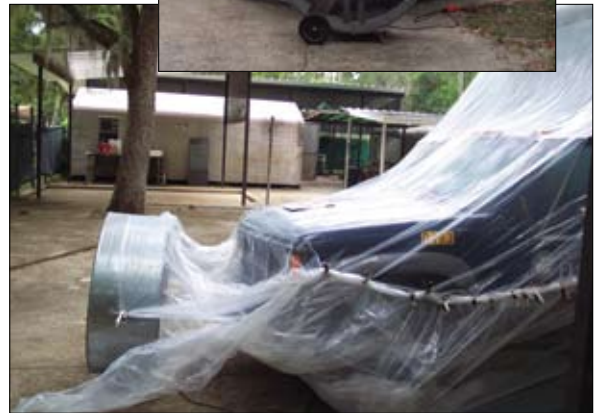
Fig. 6 and Fig. 7. A large fan used by University of Florida officials to efficiently ventilate Vikane from tarped truck during the initial aeration period. (Photos: E. Hobelmann)
