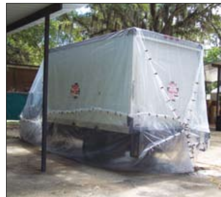
Fig. 4. A truck completely wrapped in 6-mil polyethylene for fumigation of bed bug-infested contents with Vikane gas fumigant. (Photo: E. Hobelmann)
