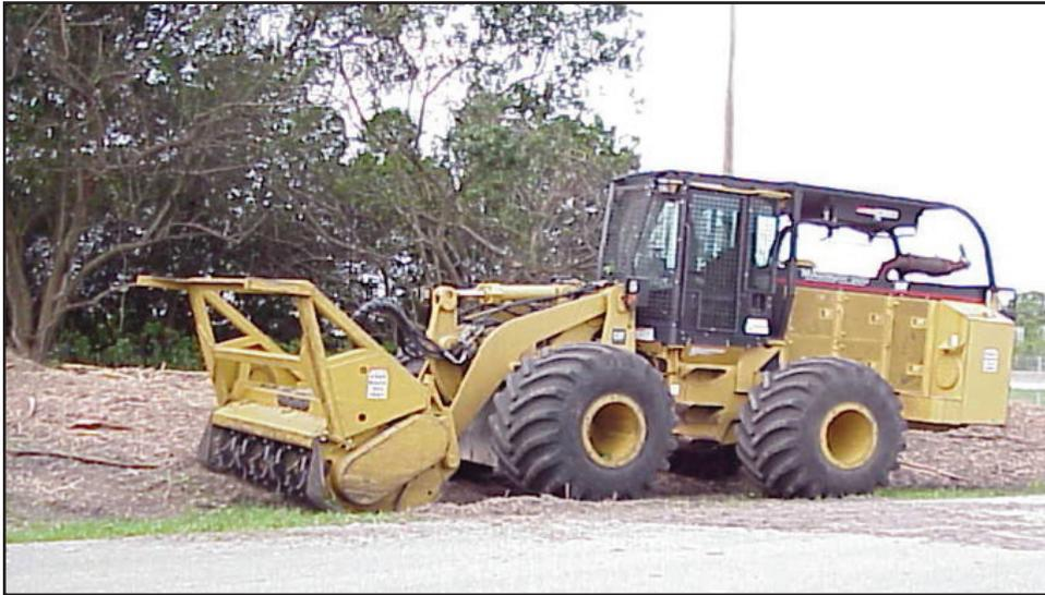
Figure 10. Front end loader in Port St. Lucie fitted with cutting/grinding attachment for removal of Brazilian peppertrees along roadside rights-of-way. (Photo credit: J. Dunton)
