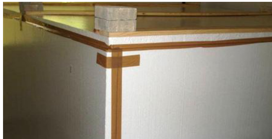
Figure 10. A "heat chamber" made of insulated polystyrene sheets built around a pile of furnishings.
