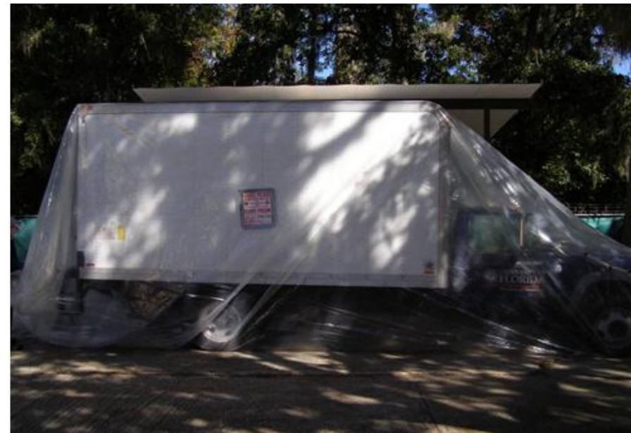
Figure 12. Fumigation chamber wrapped in polyethylene sheeting.
