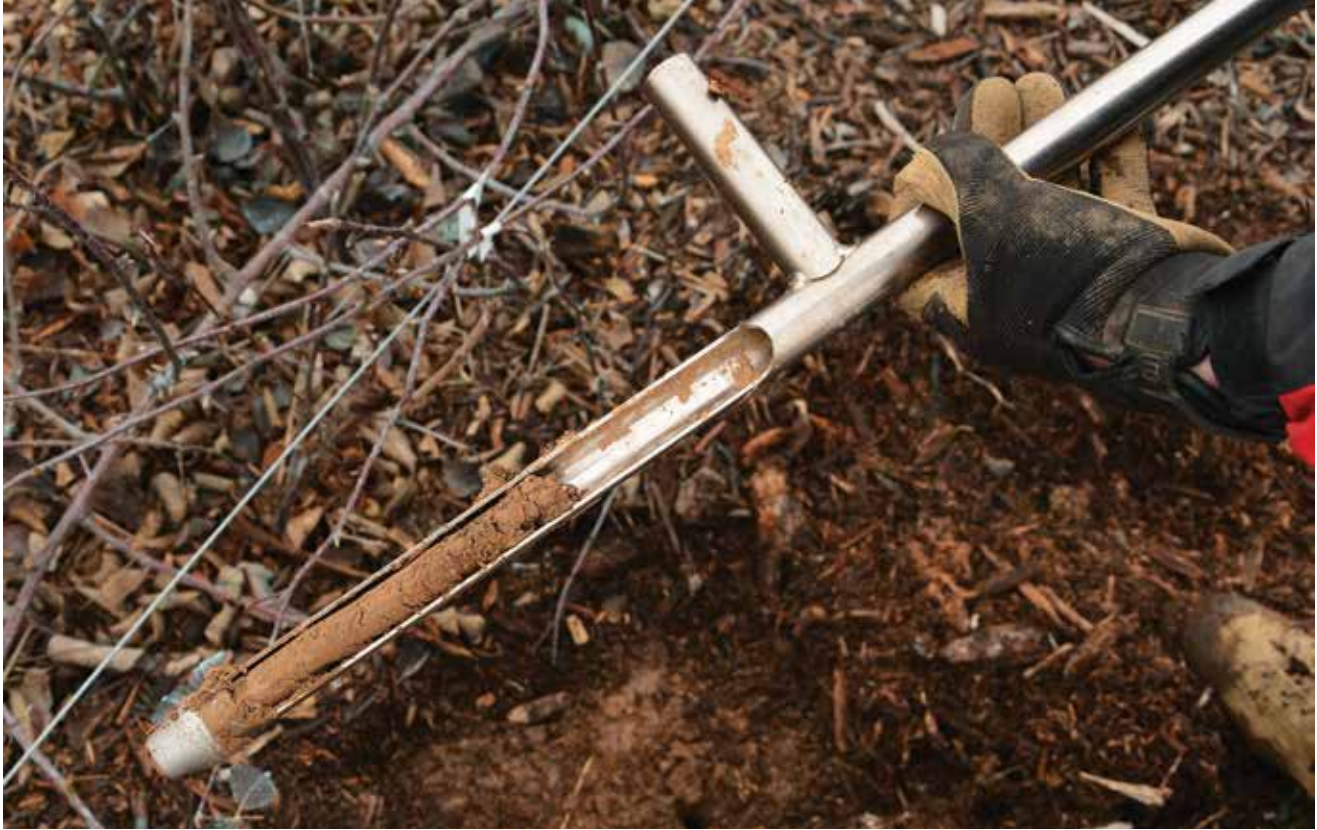
A soil probe can be used to collect multiple six-inch soil cores, which are mixed together to generate a sample. Photo by Luke Freeman.
