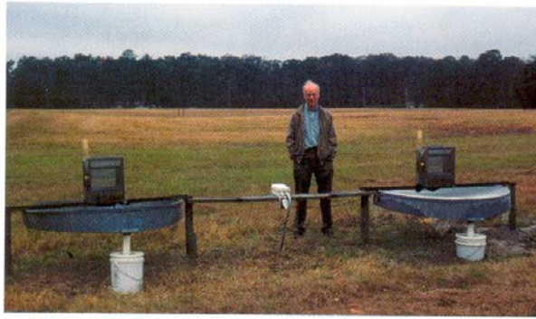
Fig. 2. A sound trap for monitoring mole cricket populations, and Tom Walker, its designer. These sound traps are in pairs (one for tawny mole crickets, one for southern mole crickets, at each location). They were operated nightly for 25 years. Photo: Lyle Buss
