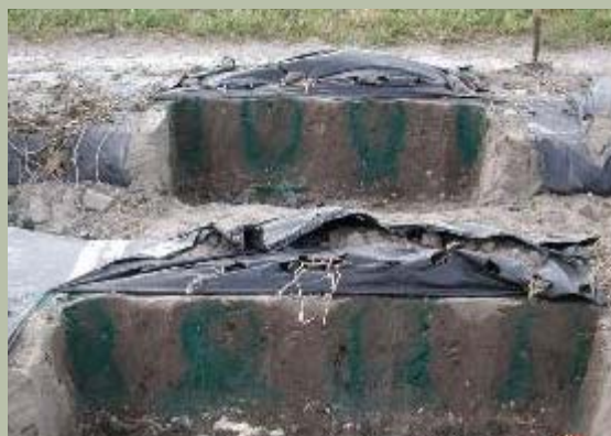
Figure 5. In seepage irrigation, water moves laterally when it reaches the spodic layer on an Acona fine sand. Photograph by: Eric Simonne.
