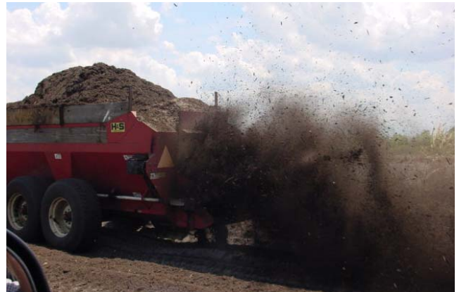
Figure 6. Broadcast application using a manure spreader. Photograph by: Monica Ozores-Hampton.
